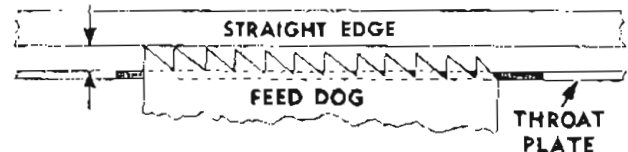
Fig. 11. Feed Dog at Correct Height
